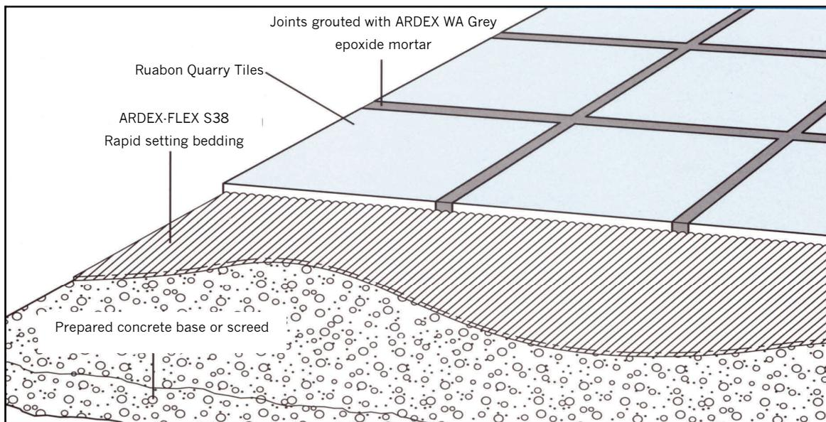
This system is recommended for industrial and high hygiene locations where the ceramic floor tiling and tile joints have to provide an impervious finish and be resistant to spillages of aggressive materials. Examples include car body workshops and showrooms, industrial process areas, battery rooms, bottling plants, abattoirs, breweries, dairies and similar food processing environments.
